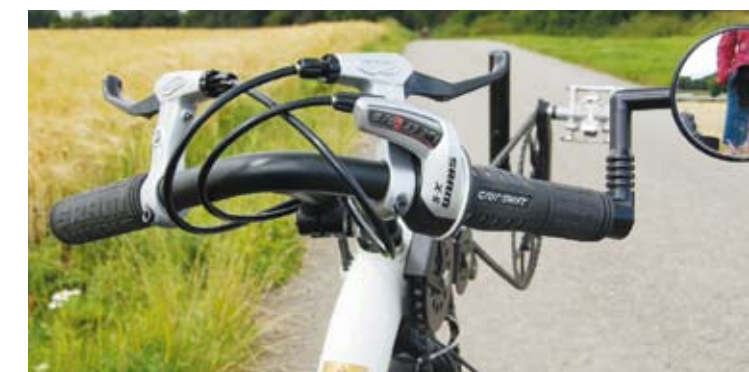
ABOVE: The front wheel drive system has remarkably little effect on the steering, while saving quite some length of chain compared to rear wheel drive equivalents.
