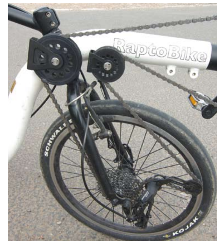
ABOVE: The front wheel drive system has remarkably little effect on the steering, while saving quite some length of chain compared to rear wheel drive equivalents.
